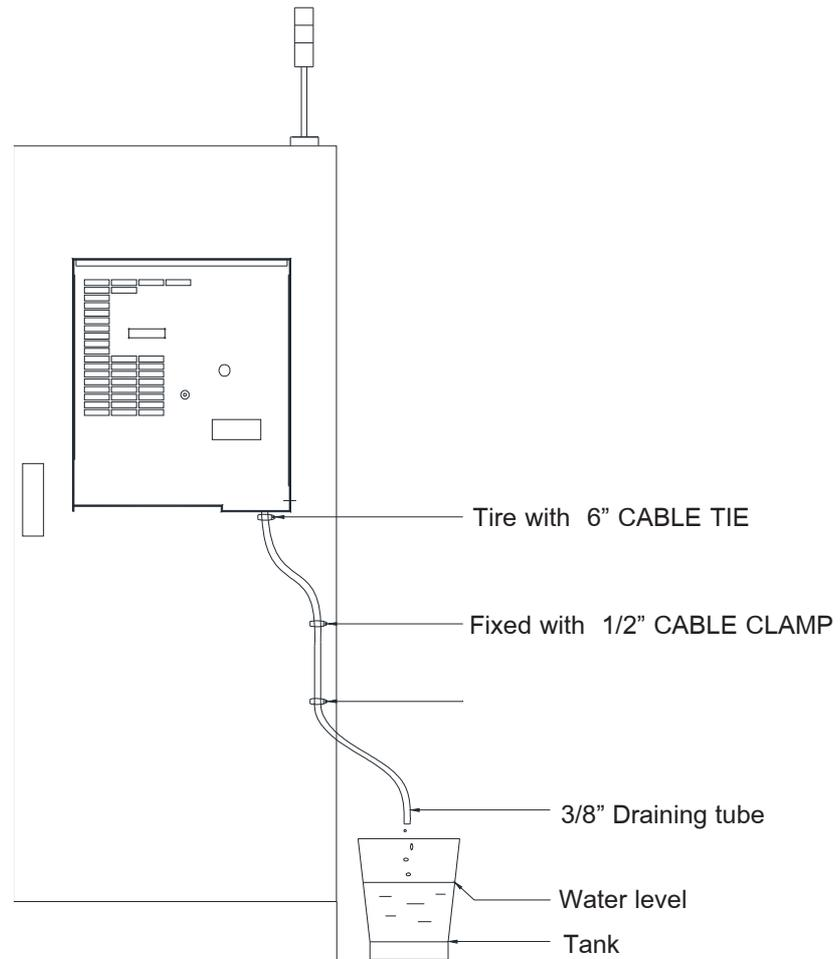
Illustrate of drainage wiring
