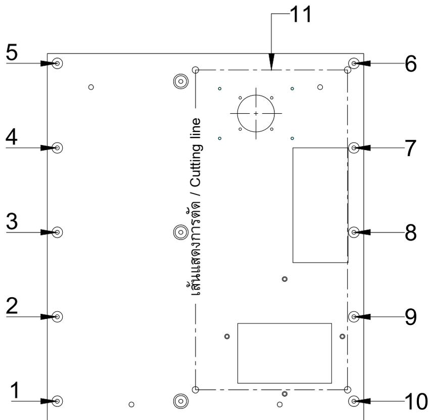
3. Cover equipments inside cabinet with clean and dry cloth, and cover with paper boxes at position will be drilled and cutted in order to prevent metal script falling in cabinet.
